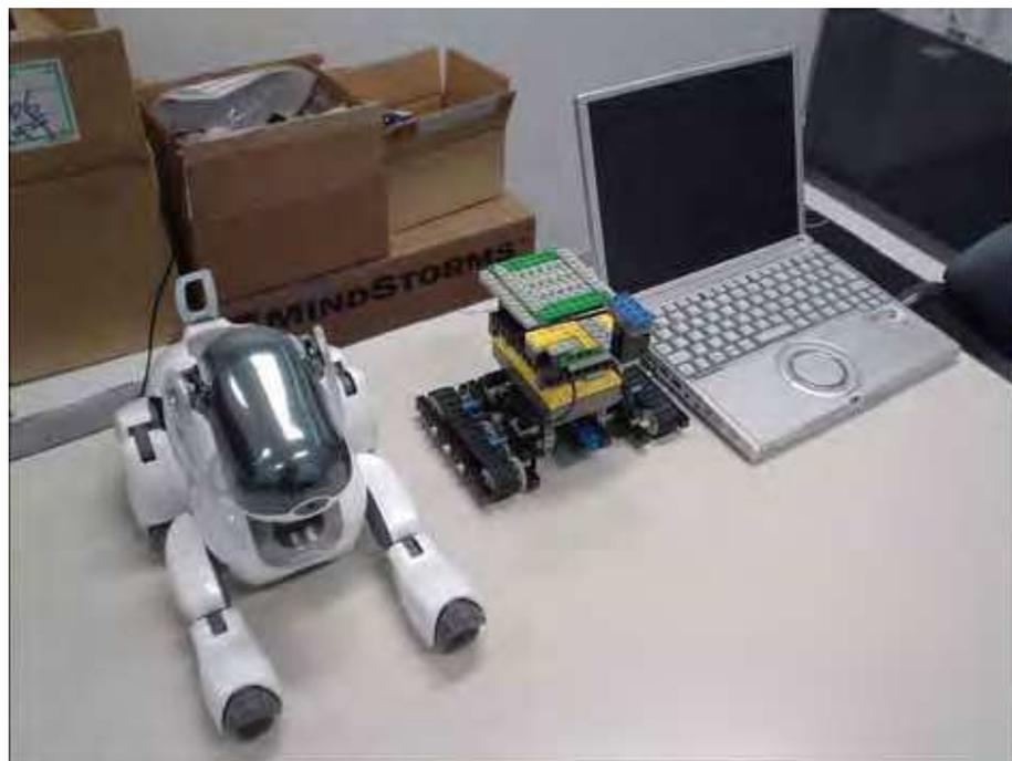
Figure 3. Two robots and a PC utilized in this experiment: AIBO, MindStorms, and a laptop PC (from left to right)
