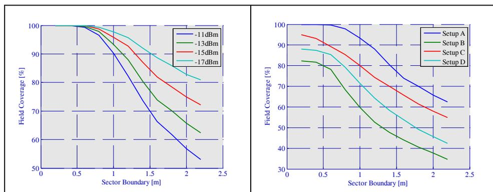
Fig. 8. (a) Field coverage associated with the dedicated section boundaries dependent of different tag sensitivity thresholds ( $-11$ ,  $-13$ ,  $-15$ , and  $-17\text{dBm}$ ) based on the pallet setup A (free-space portal area); (b) Field coverage associated with the dedicated section boundaries of all specified pallet configurations based on a sensitivity threshold of  $-13\text{dBm}$
