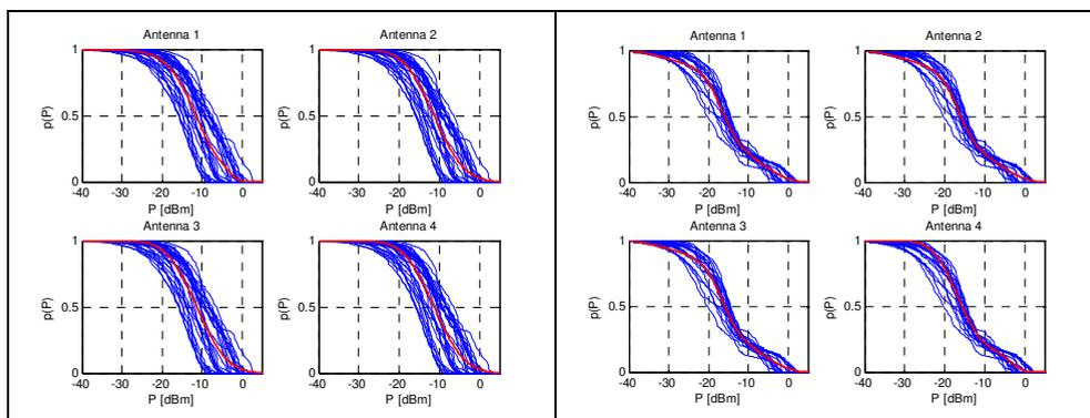
Fig. 12. (a) CDF of the used US portal derived from the FSM measurements and fitted model function showing  $p(P)$  as probability of power level greater a threshold and (b) CDF of the used EU portal derived from the FSM measurements and fitted model function showing  $p(P)$  as probability of power level greater a threshold.
