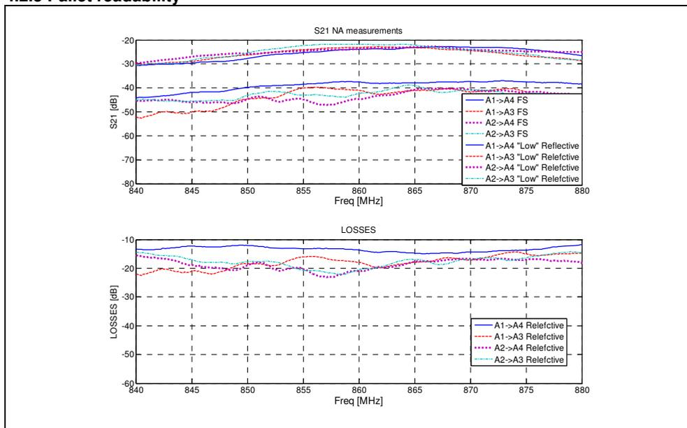
Fig. 14.  $S_{21}$  measurement results of a pallet with dimensions 1.2m x 1.4m x 2.2m by using opposite antenna pairs for radiation and reception. A network analyzer is used to determine  $S_{21}$  versus frequency.
