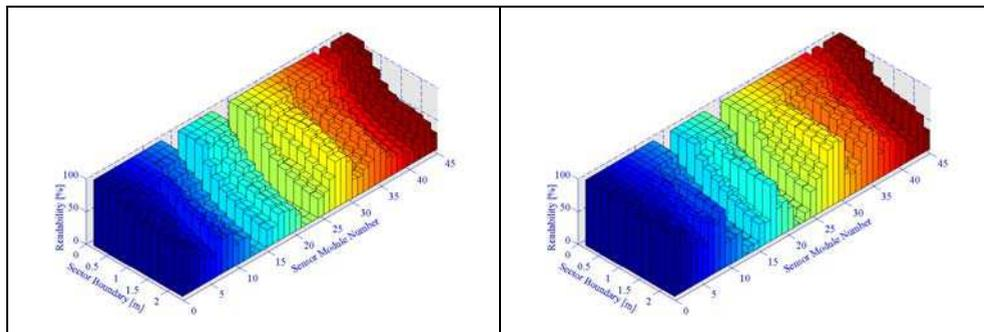
Fig. 10. (a) Readability at the position of all sensor modules of pallet setup B with a sensitivity threshold of (a)  $-13\text{dBm}$  and (b)  $-15\text{dBm}$  associated with the dedicated section boundaries (read zones)
