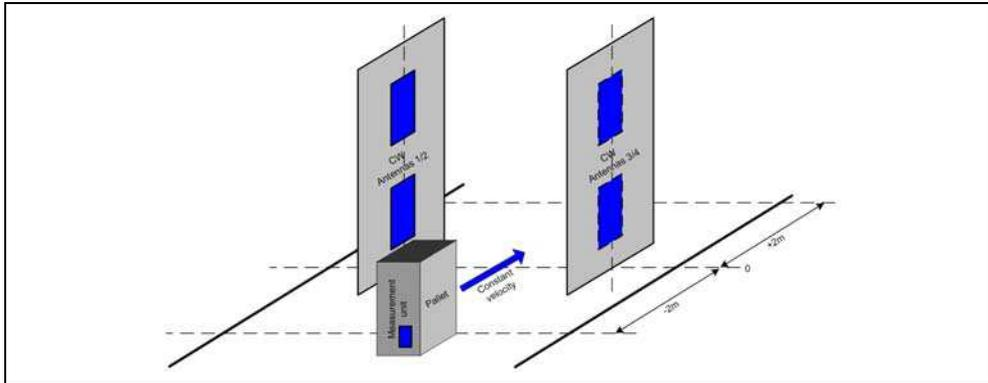
Fig. 2. Laboratory setup for interogation zone sensing. The pallet under test is passed through the portal with constant velocity by using an automated transport system
