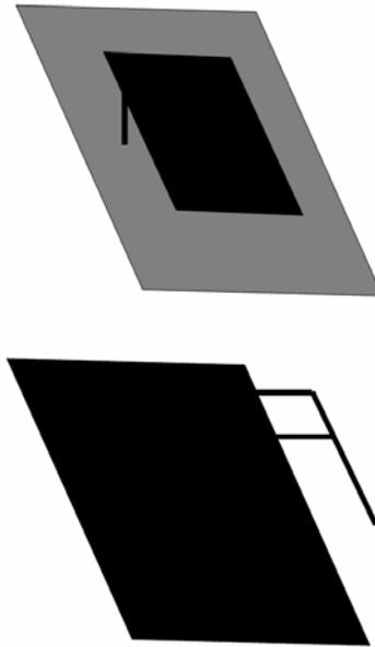
Fig. 12. Inverted-F antenna and its coplanar version
