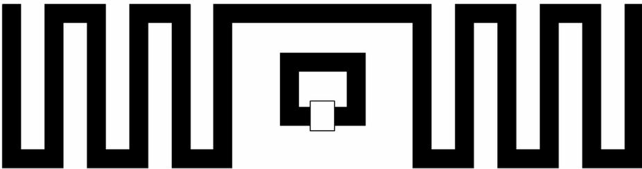
Fig. 11. Inductive loop with a meandered conducting wire
