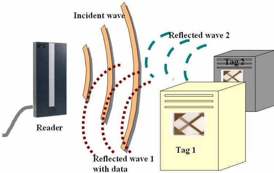
Fig. 1. Sketch of a typical RFID System
