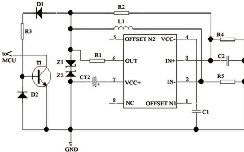
Figure 2. Structure diagram of the oscillatory circuit
