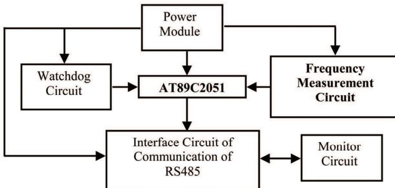
Figure 1. Block diagram of this sensor system
