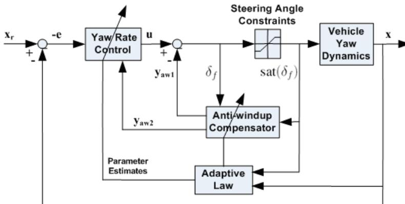
Figure 1. Adaptive control design for constrained vehicle yaw dynamics
