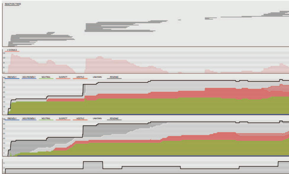
Figure 6. The cognitive task load and performance monitor describes (from lower to upper graph): the subjective workload over time, the human world view over time, the machine world view over time, the number of tracks (in gray) in combination with the number of signals (in red) over time (a performance measure), and reaction times represented using the start and end time (another performance measure)
