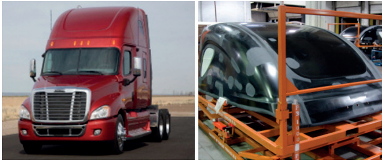
Figure 14. Glass fiber-reinforced composite body panels for truck and car [63].
