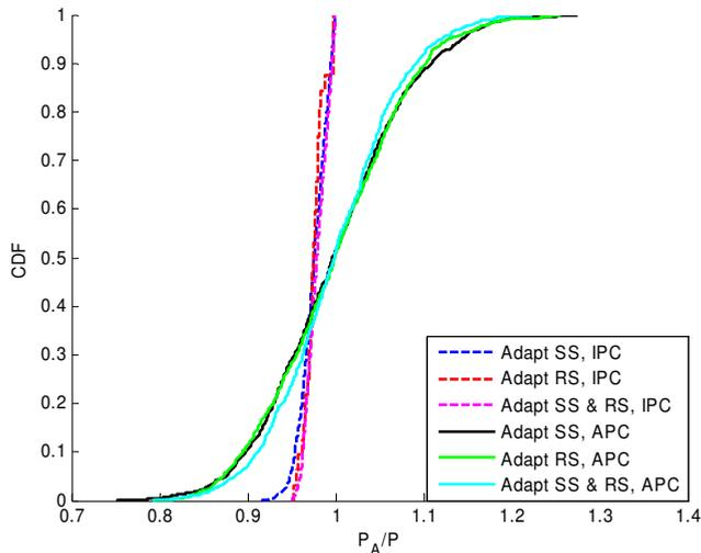
Fig. 15. CDF of total power for the solutions when  $D_{SR}=0.5$  and  $SNR=20\text{dB}$
