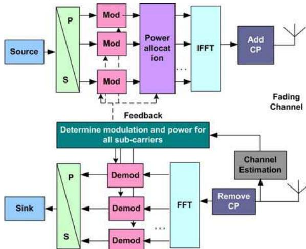
Fig. 1. Block diagram for OFDM with link adaptation
