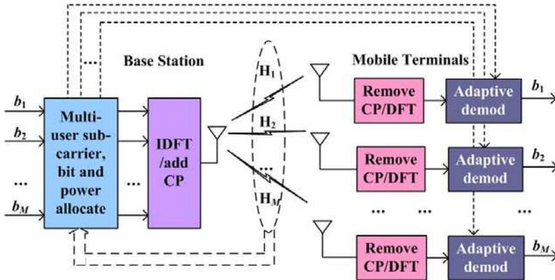
Fig. 5. A typical multi-user adaptive OFDM downlink
