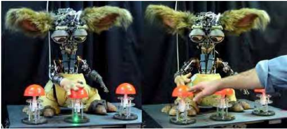
Figure 8. Leonardo activating the middle button upon request (left) and learning the name of the left button (right) (Breazeal, Brooks et al. 2003.)
