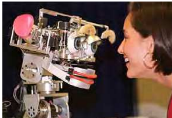
Figure 7. Kismet showing facial expressions present in human communication (Breazeal, Edsinger et al. 2001)
