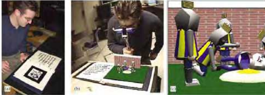
Figure 11. MagicBook with normal view (left), exo-centric view AR (middle), and immersed ego-centric view (right) (Billinghurst, Kato et al. 2001)
