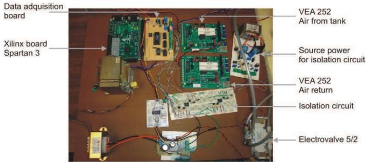
Fig. 9. Hardware used for flexible manipulator control.
