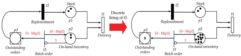
Fig. 2. An inventory control system (discrete firing example)
