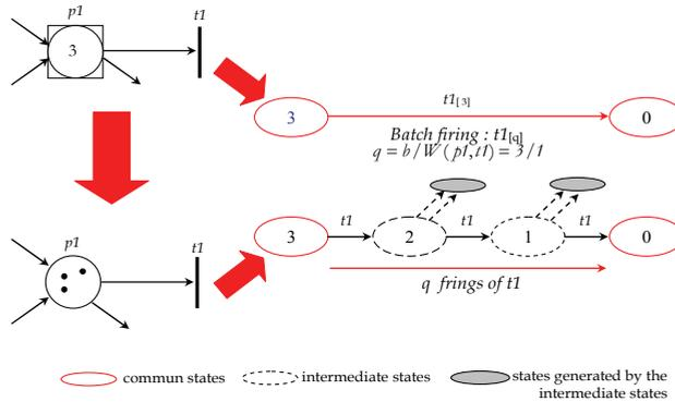
Fig. 12. Common and intermediate states of a BDSPN and its associated discrete Petri net
