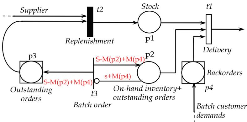
Fig. 8. BDSPN model of an inventory control system: a model that is not transformable
