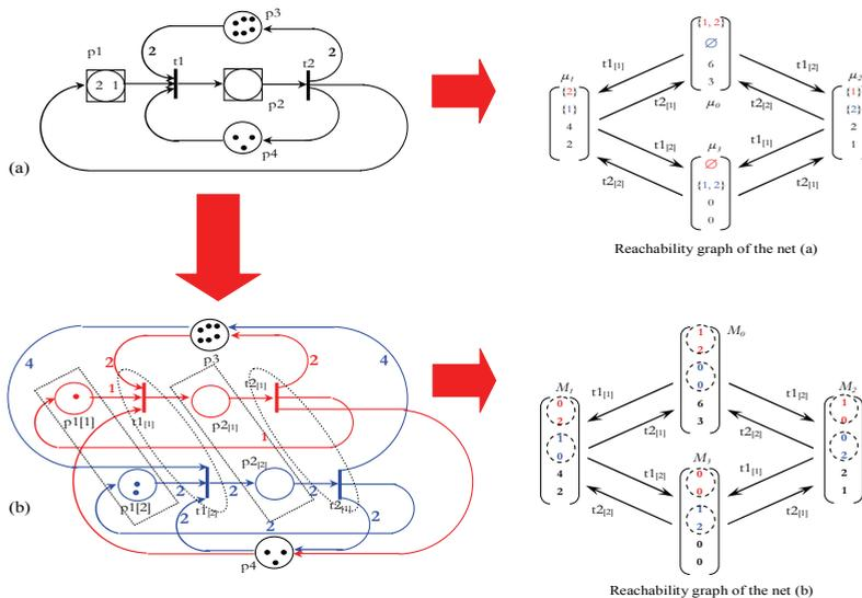
Fig. 5. Transformation of a BDSPN into an equivalent classical Petri net (general case)
