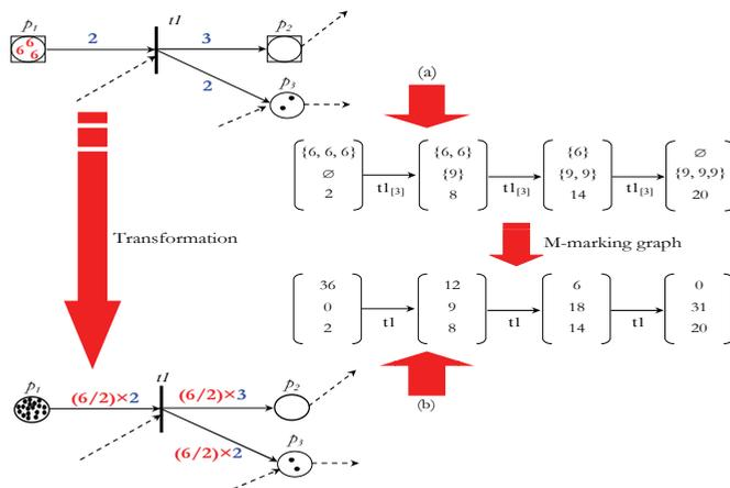
Fig. 4. Transformation of a BDSPN into an equivalent classical Petri net (special case)
