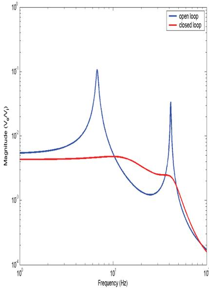
Fig. 20. Open and closed loop frequency responses of the smart beam
