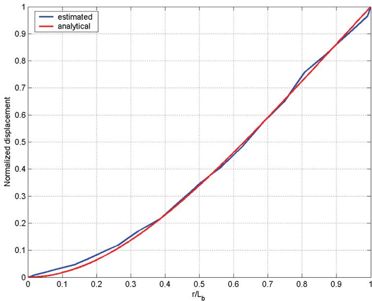
Fig. 11. First mode shape of the smart beam
