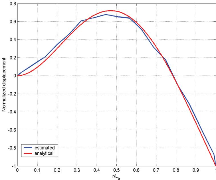
Fig. 12. Second mode shape of the smart beam
