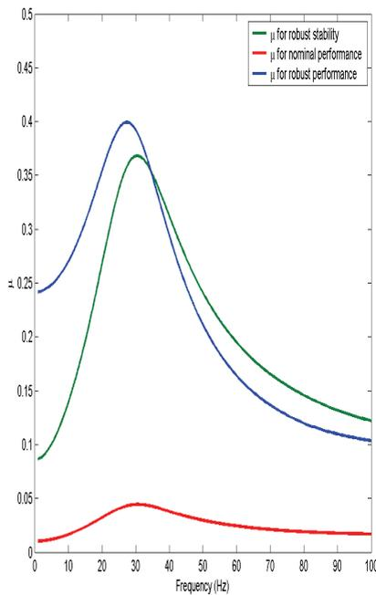
Fig. 23.  $\mu$ -analysis for spatial  $H_\infty$  controller
