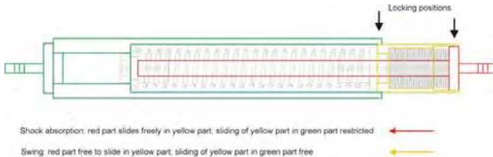
Fig. 19. Functioning of the actuator on the knee joint.
