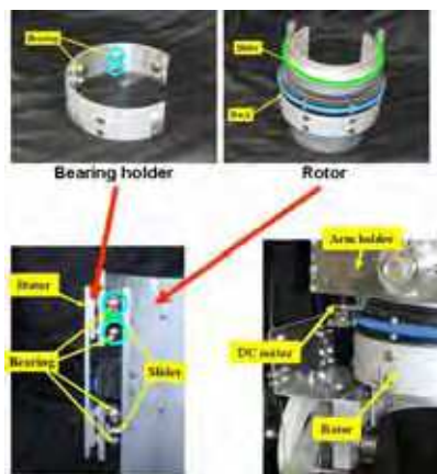
Fig. 2 Mechanism for shoulder inner/outer rotation motion assist.
