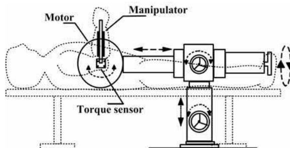
Fig. 1. Schematic diagram of a Spasticity.
