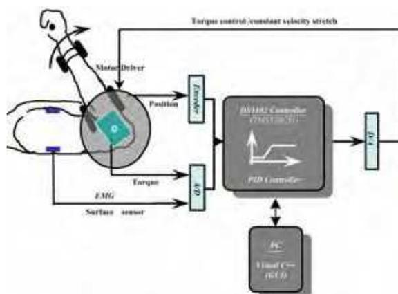
Fig. 6. Single-axis rehabilitation robot.
