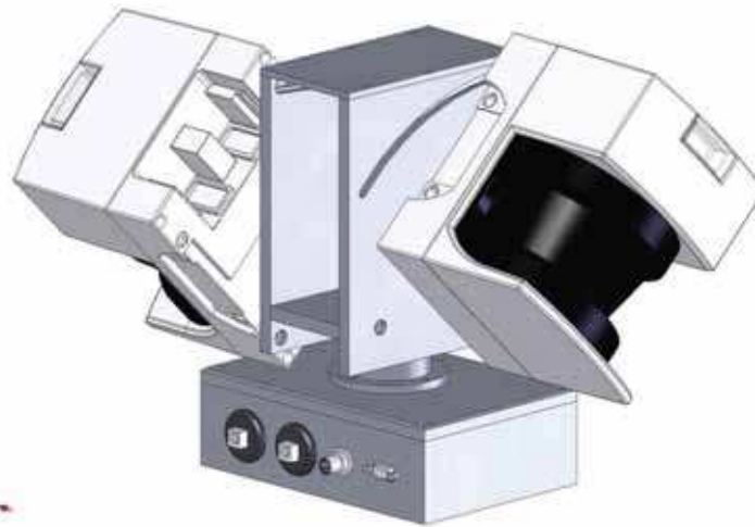
Fig. 7. CAD drawing of the new 3D Scanner
