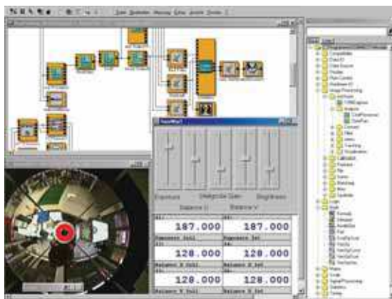
Fig. 8. ICONNECT programming environment with graph, GUI and module library
