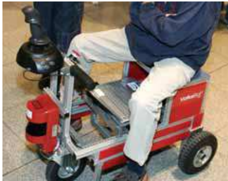
Fig.15. PeopleMover, a prototype of an intelligent vehicle on VolksBot basis
