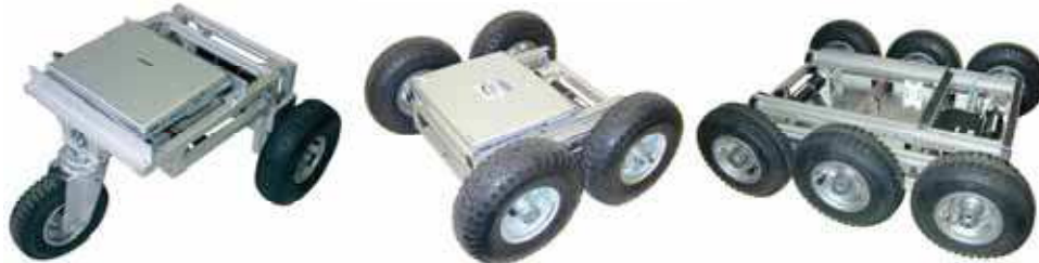
Fig.10. 3-wheeled, 4-wheeled and 6-wheeled variant of VolksBot RT
