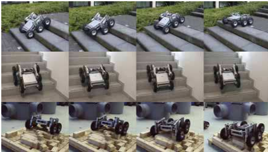
Fig. 13. VolksBot XT climbing mildly inclined stairs outdoors, a steep staircase indoors and moving over a random step field
