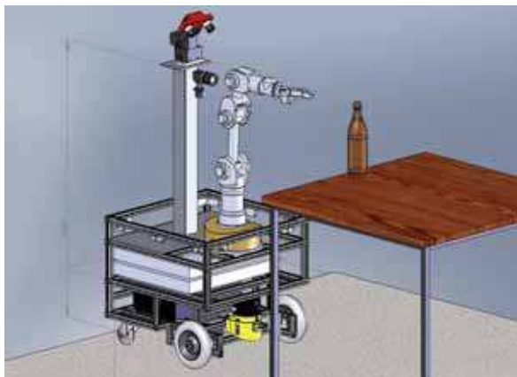
Fig.15. CAD model of the @Home VolksBot with integrated laser range finder, stereo camera and a Katana arm
