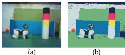
Fig. 7. (a) Image taken by the robot's camera. (b) The result of color classification of (a)
