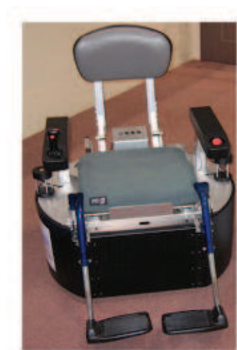
Fig. 5. The developed omnidirectional wheelchair
