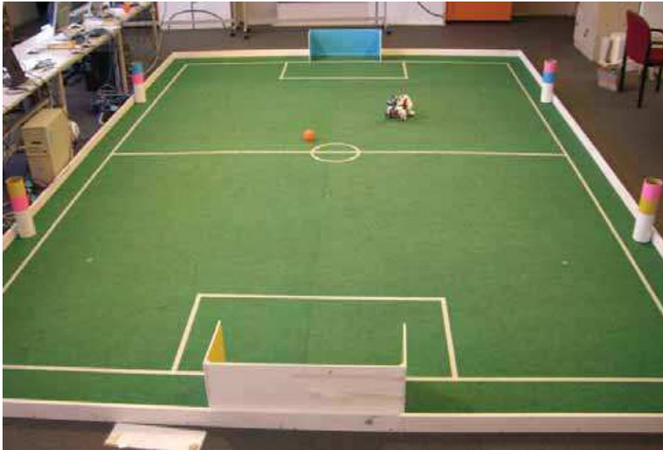
Fig. 1. A Sony AIBO ERS-7 wearing the red team uniform and the orange ball on the RoboCup four-legged league field. Note the coloured goals and localisation beacons. The outer wall is optional
