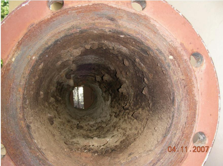
Figure 2. Photography showing the fouling layer formed in a duct section that transports crude oil (Petrobras-BR)
