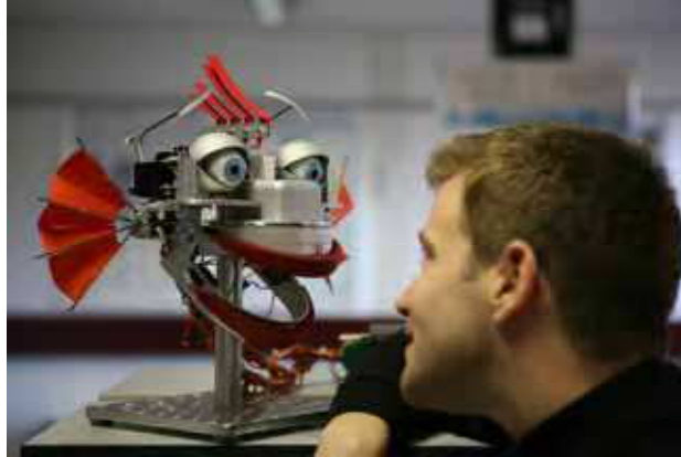
Figure 1. Robot head EDDIE with actuated features for displaying facial and non-facial expressions (Sosnowski et al., 2006a)
