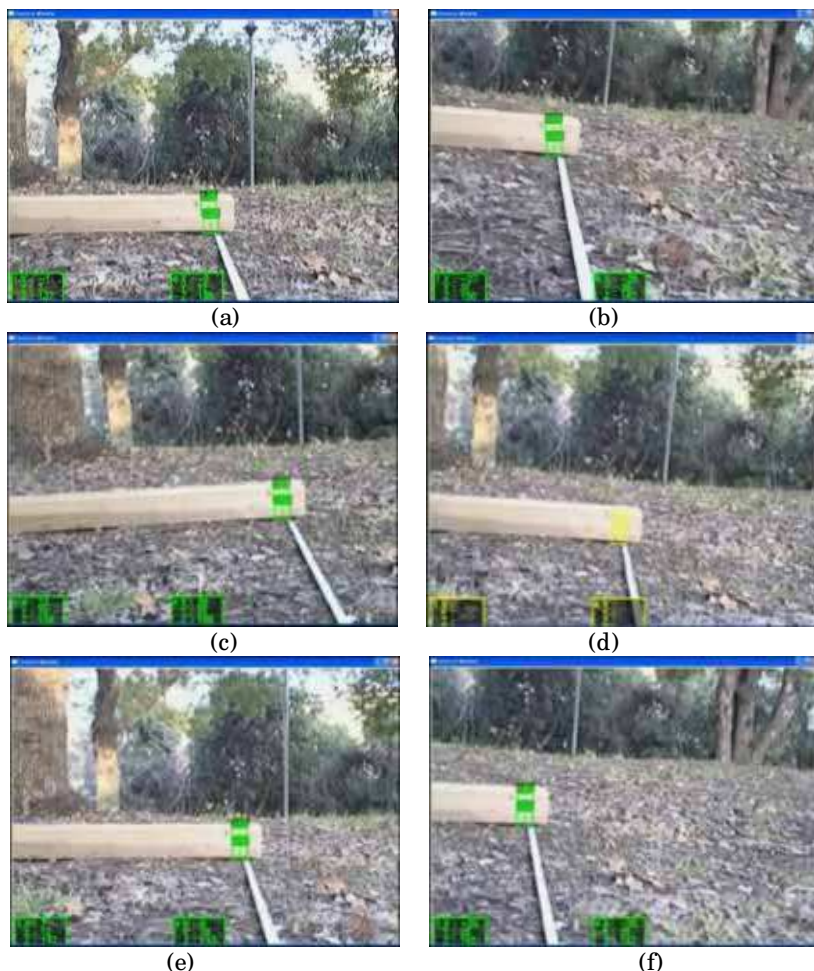
Fig. 14. Execution results of the proposed algorithm for simultaneous execution of the tracking and the stereo matching. Two small windows at the center part of images are shown the tracking windows, and the windows at the bottom of the images are shown parameters of the tracking points. The target points were not lost though the camera system was intensely shaken for five seconds. Although the stereo matching failed on two frames (the color of target window changed to yellow as shown in (d)), the distance measurement succeeded in almost all frames.
