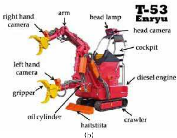
Fig. 1. Rescue robots: (a) T-52 Enryu, height: 3.45 [m], width: 2.4 [m], length: 3.5 [m] (maximum length: 10 [m]), weight: 5 [t]; and (b) T-53 Enryu, height: 2.3 [m], width: 1.4 [m] (maximum length: 7.23[m]), length: 2.32 [m], weight: 2.9 [t].
