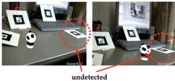
Fig. 10. Failure of marker detection even though it is captured in the image
