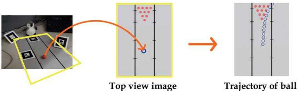
Fig. 22. Transform the ball's position to top-view image
