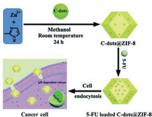
Figure 8. Schematic representation of the synthetic route of the C-dots@ZIF-8 for simultaneous anticancer drug delivery and fluorescence imaging of cancer cell (image from He et al. [67])—Copyright © 2014, Royal Society of Chemistry).
