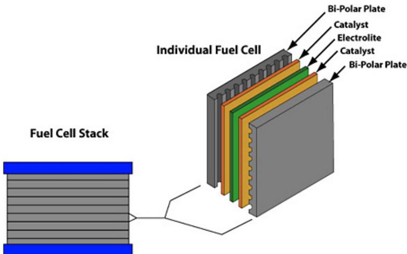
Figure 2. Showing components of fuel cell stack (www.tech-etech.com)
