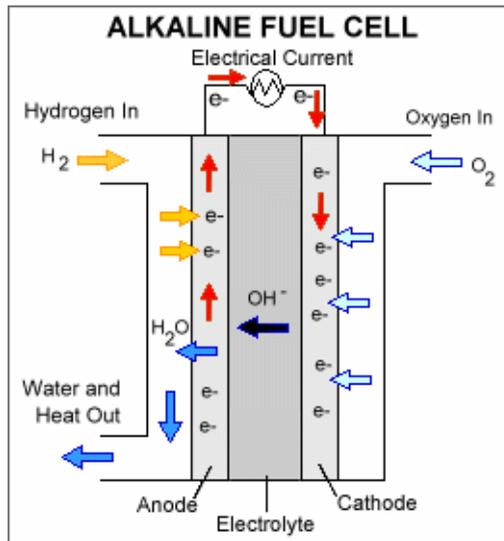
Figure 4. Showing components of alkaline fuel cell (www.fuelcellmarkets.com)
