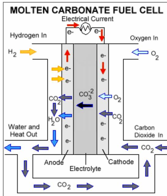
Figure 6. Showing components of molten carbon fuel cell ([www.fuelcellmarkets.com](http://www.fuelcellmarkets.com))
