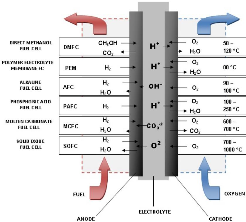
Figure 3. Showing different types of fuel cells ([www.fuelcells.org](http://www.fuelcells.org))
