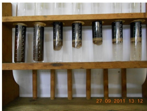
Figure 3. Stability bottle test of water-in-crude-oil emulsion (Silva, 2012).
