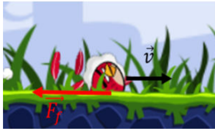
Figure 5. We can see that force friction is working in the opposite direction of the bird, causing the bird to slow down.
