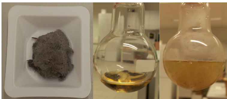
Figure 14. One-step dissolution and hydrolysis of fiber sludge (left) using tailored ionic liquid (middle, tailored IL and fiber sludge) and regeneration of cellulose (right).
