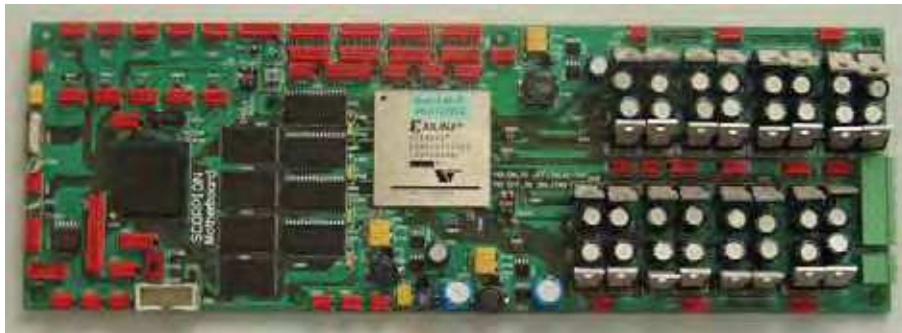
Fig. 9. SCORPION control board featuring an MPC555 and a Xilinx Virtex E FPGA
