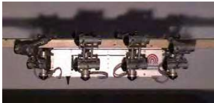
Fig. 20. SCORPION Robot using the PCR approach to climb along a beam
