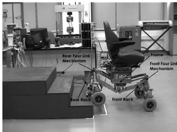
Figure 10. Prototype designed
