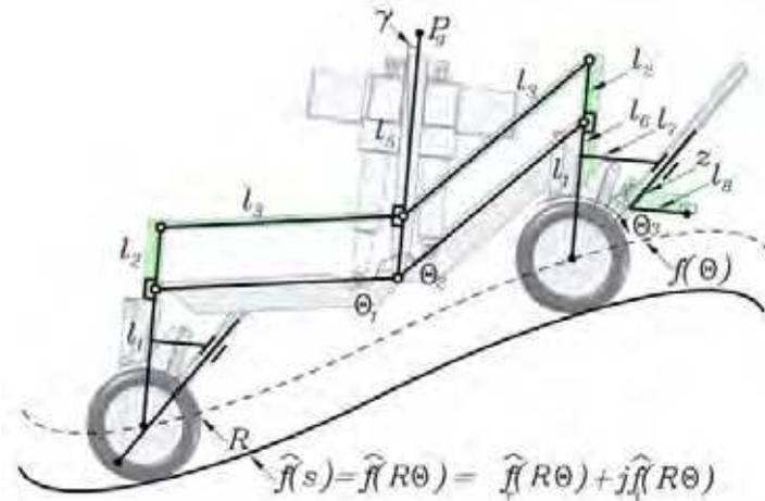
Figure 9. Wheelchair kinematics diagram
