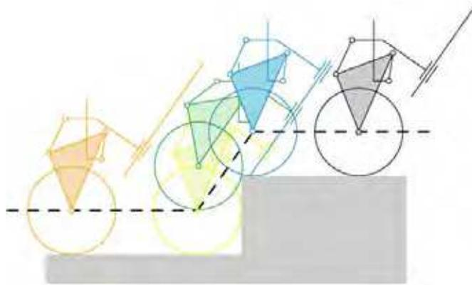
Figure 6. Trajectory of the climbing mechanism when overpass an obstacle
