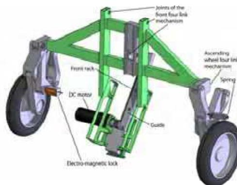
Figure 2. Climbing Mechanism Designed
