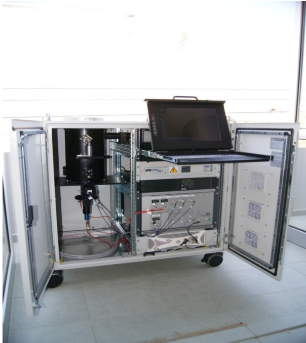
Figure 3. CUT's Depolarization Lidar System
