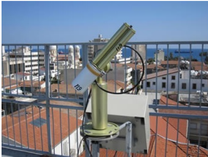
Figure 1. CUT-TEPAK AERONET station
