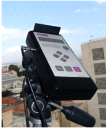
Figure 2. MICROTOPS II handheld sunphotometer
