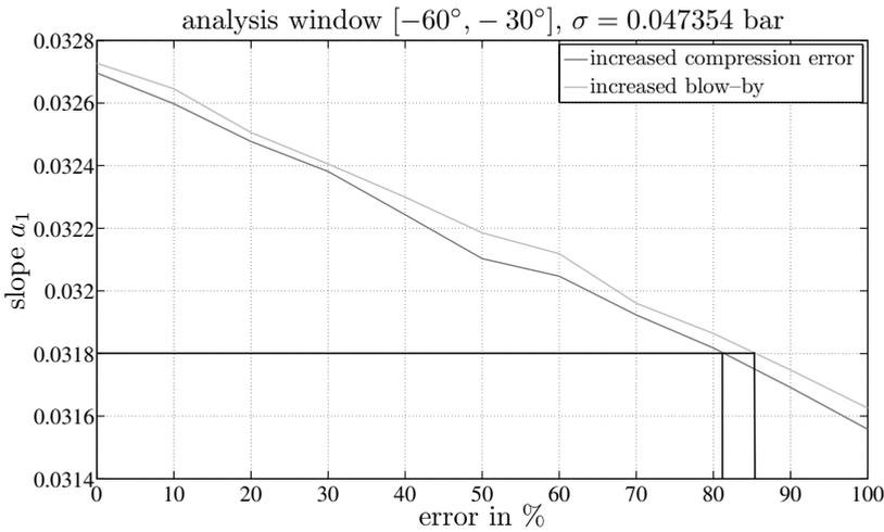
**Figure 5.** Slope parameter  $a_1$  for the lower analysis window  $[-60^\circ, -30^\circ]$  to TDC ( $a_1 = 3.180 \times 10^{-2}$ ). The lines for compression and blow-by error are still too close together for a separation of the failure modes.
