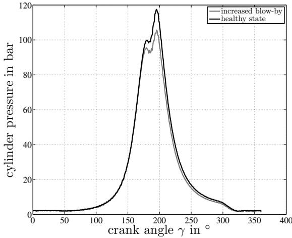
**Figure 10.** Measured cylinder pressure representing a *healthy state* and one cylinder with increased blow-by of a different engine. The sources of defect were in both cases documented by the manufacturer after disassembly of the machine.
