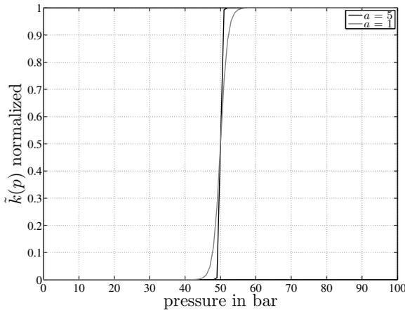
**Figure 1.** Sigmoid function to describe the nonlinear behavior of blow-by related to the cylinder pressure. The rapid increase of the mass passing by the cylinder results from the tear-off of the oil film at the piston crown.
