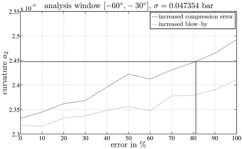
**Figure 6.** Curvature parameter  $a_2$  for the lower analysis window  $[-60^\circ, -30^\circ]$  to TDC ( $a_2 = 2.447 \times 10^{-5}$ ). Because there is only one failure mode in the allowed range  $a_2$  allows the separation between blow-by and compression error.
