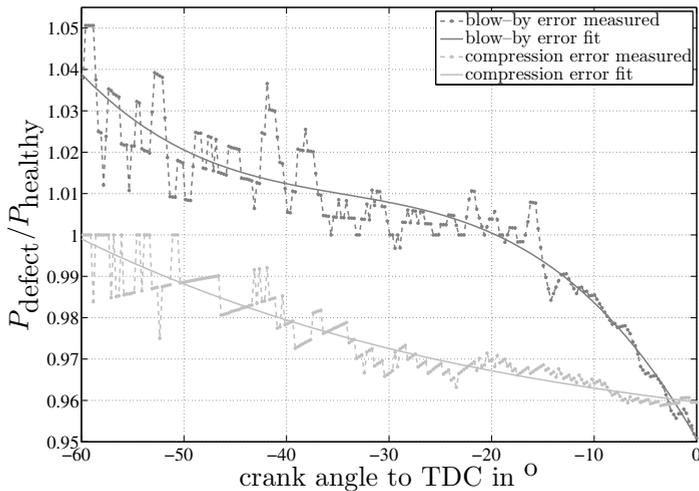
**Figure 7.** Comparison of the ratio  $P_{\text{defect}}/P_{\text{healthy}}$  for an engine showing blow-by error and compression error respectively showing different curvature in their slopes especially in the interval  $[-40^\circ, 0^\circ]$ .
