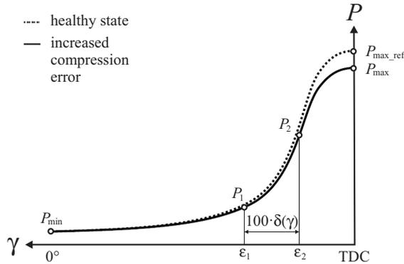
**Figure 3.** Typical cylinder pressure traces representing a *healthy state* (dashed) and a cylinder with increased compression error (solid). The analysis window  $\delta(\gamma)$  is applied within the well-defined compression phase in order to avoid the influence of combustion effects as well as measurement noise at low signal levels.
