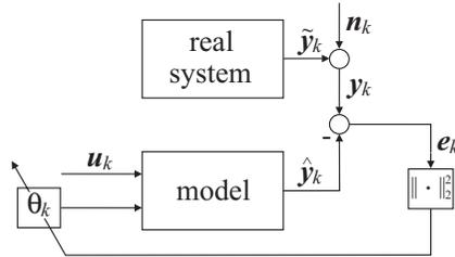
**Figure 8.** Block diagram of the parameter identification of large diesel engines. The index  $k$  indicates the iterative nature of the optimization procedure. By minimizing the residual error between measured and calculated cylinder pressure, the optimal parameter configuration for blow-by and compression ratio is found. Based on the *a priori* known limits of the parameters, the engine state can be assessed and monitored.
