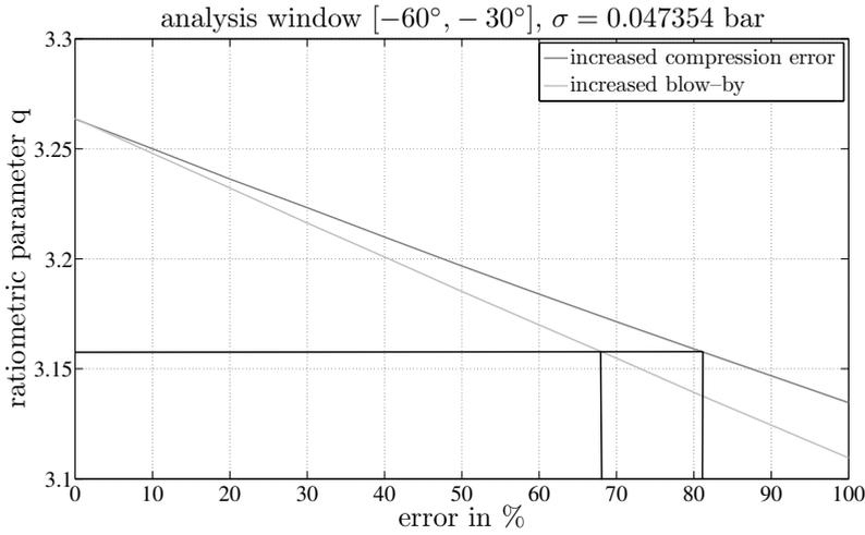
**Figure 4.** Ratiometric parameter  $q$  for the lower analysis window  $[-60^\circ, -30^\circ]$  to TDC ( $q = 3.1587$ ). The lines for compression and blow-by error are proceeding too close for a failure separation.
