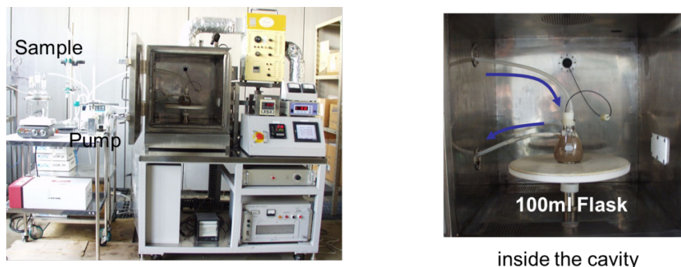
Figure 7. Microwave apparatus for continuous synthesis of ETBE (Shikoku Instrumentation Co., Ltd.)
