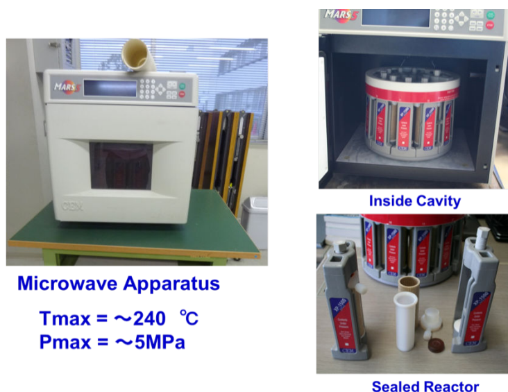
Figure 9. Microwave apparatus for pressurized synthesis of ETBE in a sealed reactor vessel (MARS5, CEM Corporation, Japan)
