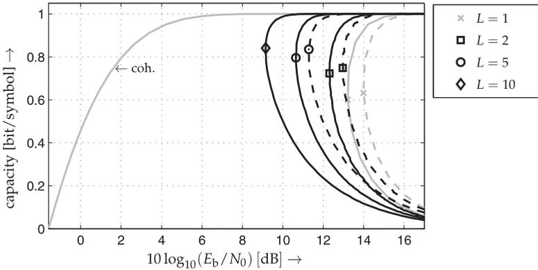
**Figure 3.** Capacity of BICM BPSK IR-UWB for soft/hard-output DD (solid gray/dashed gray), soft-output MSDD with  $L = 2, 5,$  and  $10$  (solid black), and DF-DD with  $L = 2$  and  $5$  (dashed black). Gaussian approximation with time-bandwidth product  $N = 400$ .
