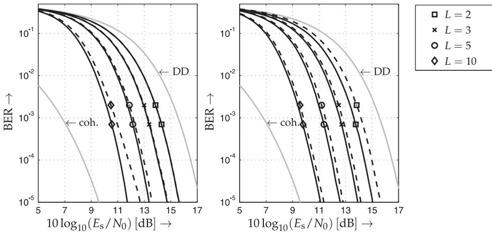
**Figure 2.** BER of uncoded BPSK IR-UWB transmission with autocorrelation-based detection with  $L = 2, 3, 5,$  and  $10$  (right to left). Solid: MSDD, dashed: DF-DD, left: processing of non-overlapping blocks, right: combining of multiple observations obtained by processing of maximum-overlapping blocks. Gaussian approximation with time-bandwidth product  $N = 400$ .
