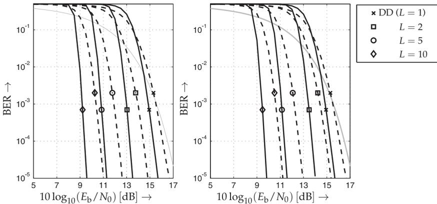
**Figure 4.** BER of convolutionally-coded BICM BPSK IR-UWB with autocorrelation-based detection with  $L = 1, 2, 5,$  and  $10$  (right to left). Solid: optimum code rate ( $R_c = 2/3$  for DD with  $L = 1$  and  $R_c = 3/4$  for  $L = 2, 5$  and  $10$ ), dashed:  $R_c = 1/2$ , gray: DD uncoded, left: soft-output MSDD, right: DF-DD, both using multiple-observations combining with maximum overlap. Gaussian approximation with time-bandwidth product  $N = 400$ .
