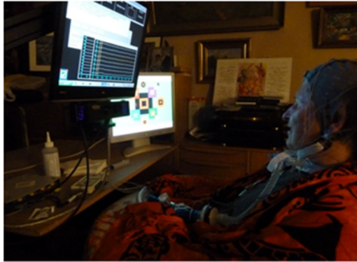
Figure 6. ALS patient at her home, after finishing her brain painting. While painting, the brain painting matrix appears on one screen while on an additional monitor, placed on the table in the background, she can follow the progress of her painting. The brain painting software is operated by the family or caregivers and requires few steps only for set up.
