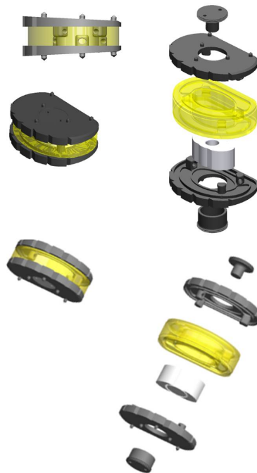
Figure 7. Second generation of lumbar ESP® ( 2005 ) : the shape of the endplates provides lordosis
