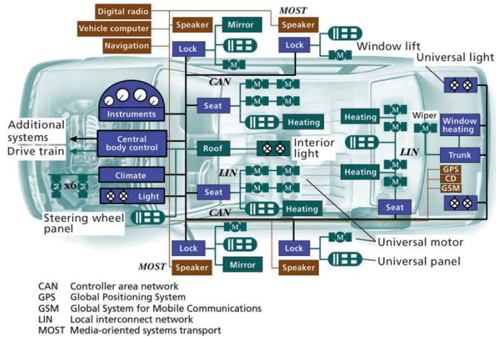
**Figure 1.** Design of a modern vehicle's network architecture, [13].
