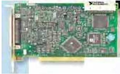
Figure 7 (a). A DAQ PCI card
