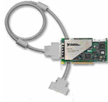
Figure 7(b). A DAQ card with cable
