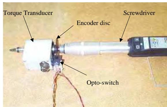
Figure 8. A screwdriver attached transducer and encoder
