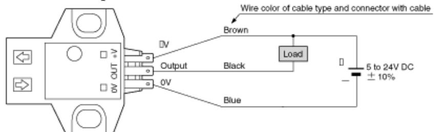
Figure 3.2 Typical wiring diagram
