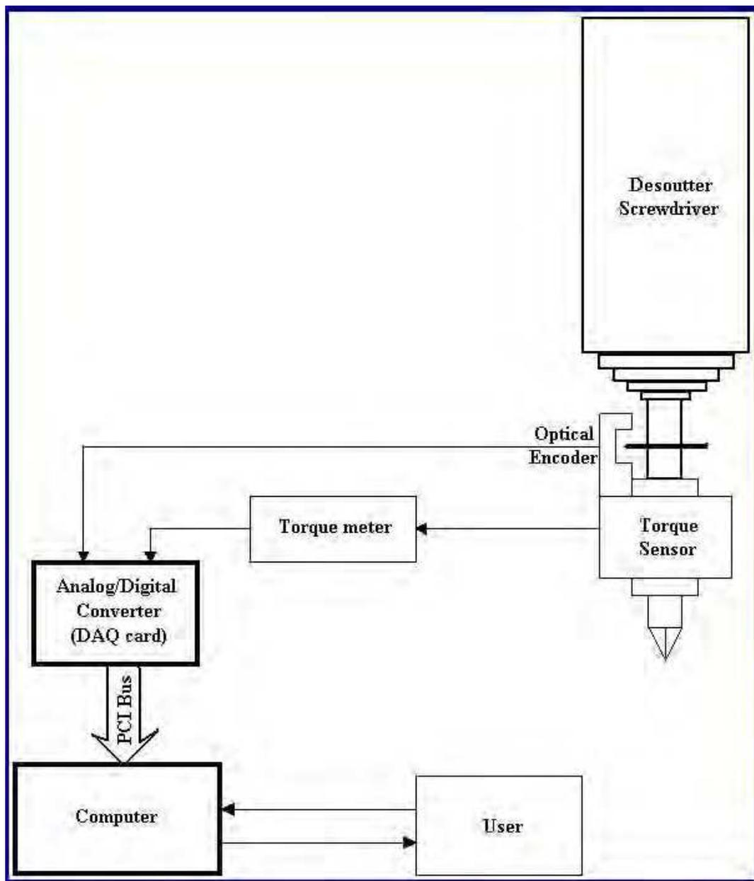
Figure 11. The overview of the experimental test rig
