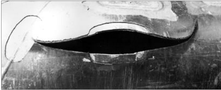
Figure 17. Burst initiated on slit B – a detail
