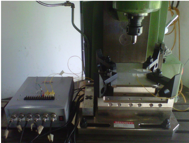
Figure 1. Friction stir welding experimental set up [5].
