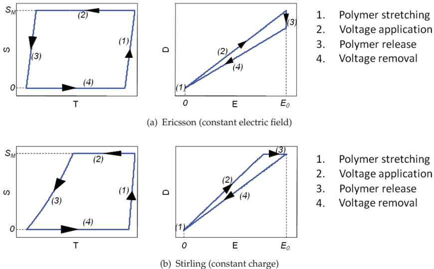
**Figure 8.** Electrostatic energy harvesting cycles and mechanical cycles for electrostrictive polymers.
