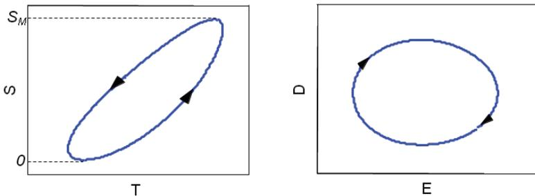
Figure 12. Energy harvesting cycle using AC pseudo-piezoelectric mode.
