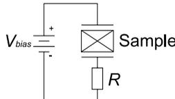
**Figure 5.** Energy harvesting circuit
