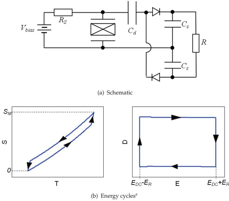
**Figure 13.** Pseudo-piezoelectric DC energy harvesting: (a) schematic; (b) energy cycles.
