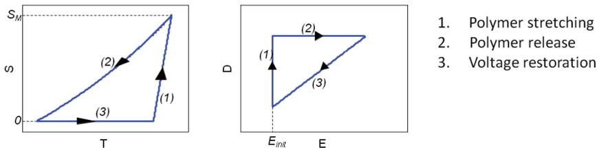
**Figure 9.** Energy harvesting cycle using hybrid Stirling/Ericsson combination.
