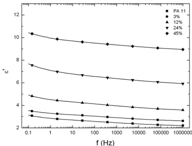
**Figure 3.** Room temperature dielectric permittivity ( $\epsilon'$ ) versus frequency for BaTiO<sub>3</sub>/Polyamide 11 composites with volume fraction ranging from 0%, to 45%.
