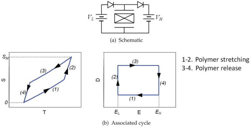
**Figure 10.** Passive energy harvesting cycle.
