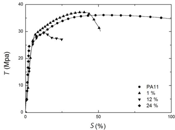
**Figure 4.** Room temperature stress versus strain measurements for BaTiO<sub>3</sub>/Polyamide 11 composites with volume fraction ranging from 0%, to 24%.
