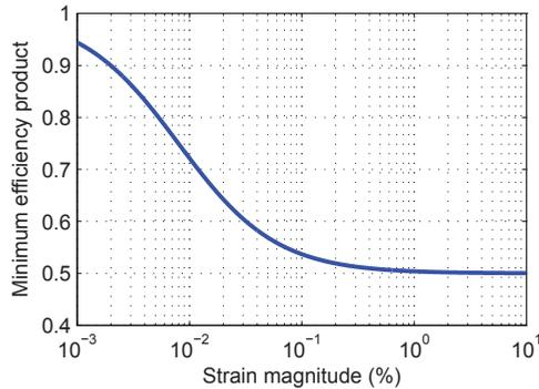
**Figure 17.** Minimum product of the injection and extraction efficiencies as a function of the strain for polyurethane *PS* 2000 material ( $M_{31} = 5 \times 10^{-18} \text{ m}^2 \cdot \text{V}^{-2}$ ;  $\epsilon_{33}^S = 6.1\epsilon_0$ ;  $Y = 33.8 \text{ MPa}$  - [49]).
