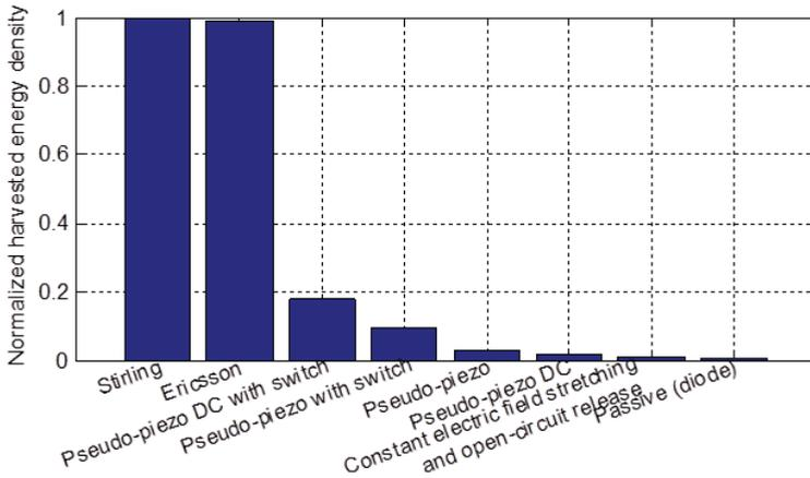
**Figure 16.** Maximum energy density (normalized with respect to the maximum one) of the energy harvesting techniques ( $\gamma = 0.8$  for the nonlinear processing techniques).
