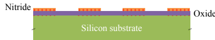
Figure 35. Patterned SiO 2 /Si 3 N 4 electrets from IMEC and used in a structure [45].
