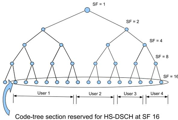
**Figure 1.** Orthogonal Variable Spreading Factor (OVSF) code tree.
