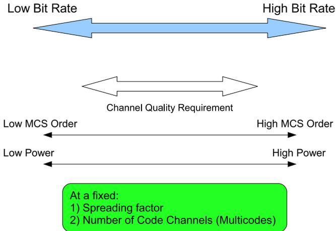
Figure 2. Bit rate and channel quality requirement trade-off for HSDPA.
