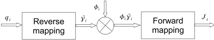
**Figure 6.** The conversion process from the received CQI,  $q_i$ , from the mobile to the assigned rate index  $J_i$  at the base station. ([14]©IET)
