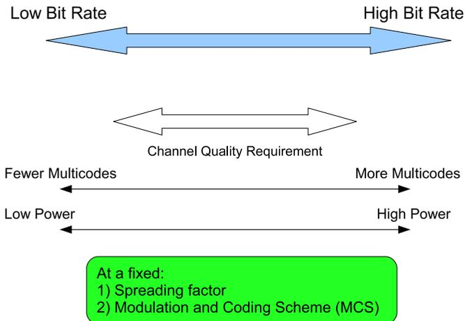
Figure 3. Bit rate and channel quality requirement trade-off for HSDPA.
