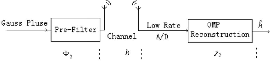
**Figure 3.** The FIR filtering matrix estimation
