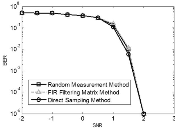
**Figure 8.** The BER performances of three estimation methods with noiseless UWB signals
