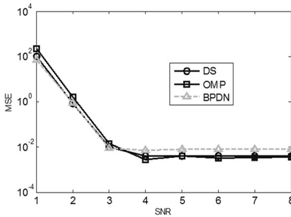
**Figure 10.** The comparison of the mean square error for the three reconstruction algorithms
