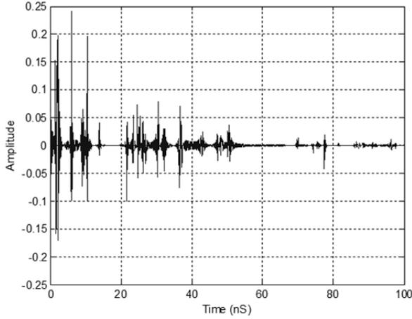
**Figure 4.** Impulse response of the UWB channel
