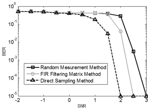
**Figure 9.** The BER performances of three estimation methods with noisy UWB signals
