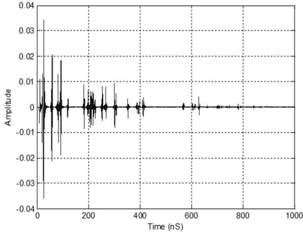
**Figure 5.** Gaussian pulse response of the UWB channel
