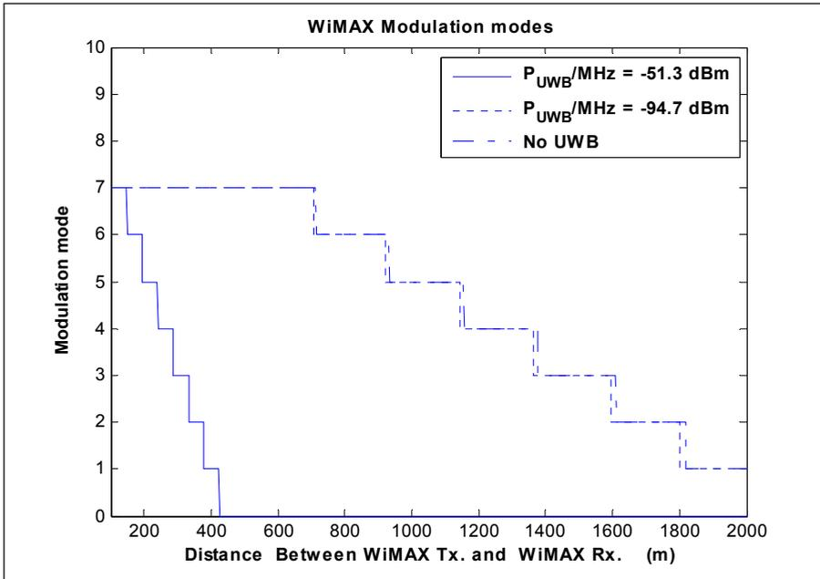
**Figure 5.** 2.5 GHz WiMAX modulation modes for different UWB power densities with a 1 m distance between the UWB transmitter and the WiMAX receiver assuming a WiMAX transmitted power of 40 dBm/sector.
