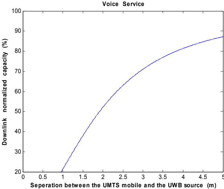
Figure 11. Effect of the UWB interference on the macrocell normalized capacity as a function of the separation between the UWB transmitter and the UMTS mobile ( $P_{UWB} = -60\text{ dBm/MHz}$ ).
