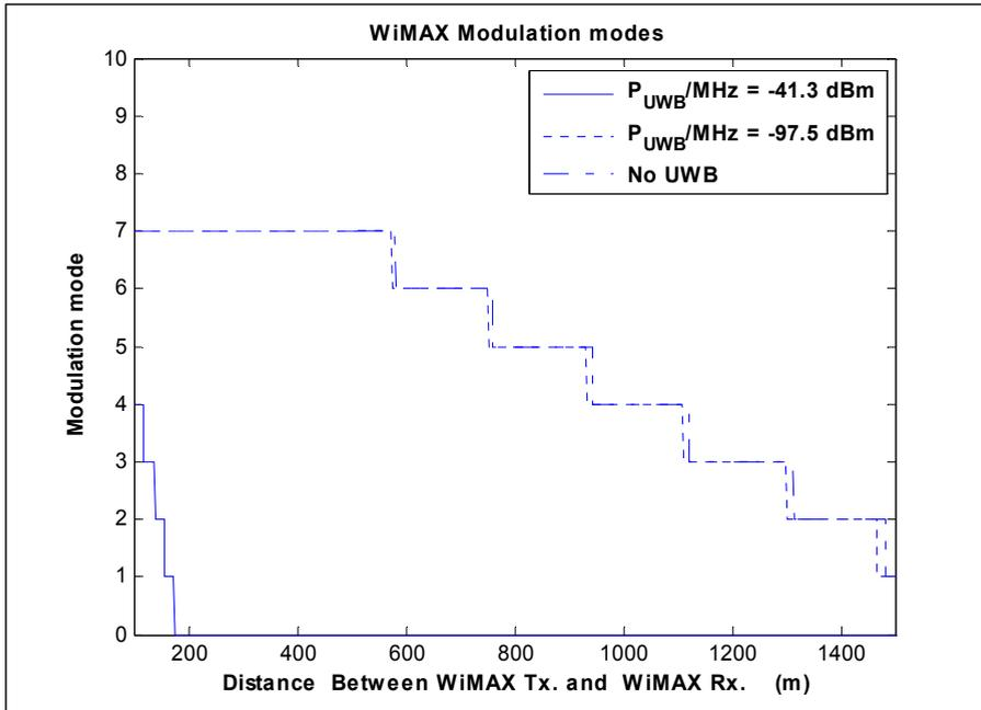
**Figure 6.** 3.5 GHz WiMAX downlink modulation modes versus distance between the WiMAX transmitter and receiver, for different UWB power densities from 4 UWB transmitters at 1 m distance to the WiMAX receiver and assuming a WiMAX transmitted power of 40 dBm/sector.
