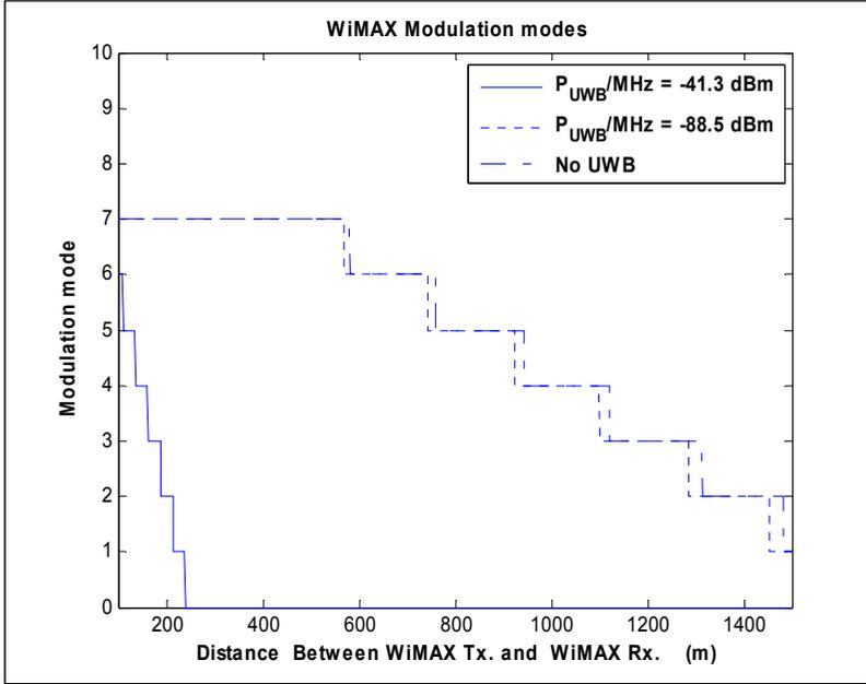
**Figure 2.** 3.5 GHz WiMAX modulation modes for different UWB power densities with a 1 m distance between the UWB transmitter and the WiMAX receiver assuming a WiMAX transmitted power of 40 dBm/sector.
