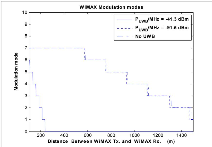
**Figure 4.** 3.5 GHz WiMAX modulation modes for different UWB power densities with a 1 m distance between the UWB transmitter and the WiMAX receiver assuming a WiMAX transmitted power of 40 dBm/sector.
