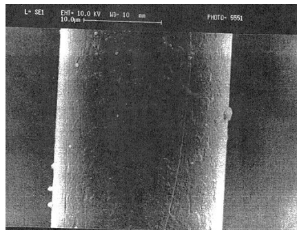
Figure 22. SEM micrograph of PET sample treated with 5% ammonium hydroxide, at room temperature, 120 days, under relax condition [91].
