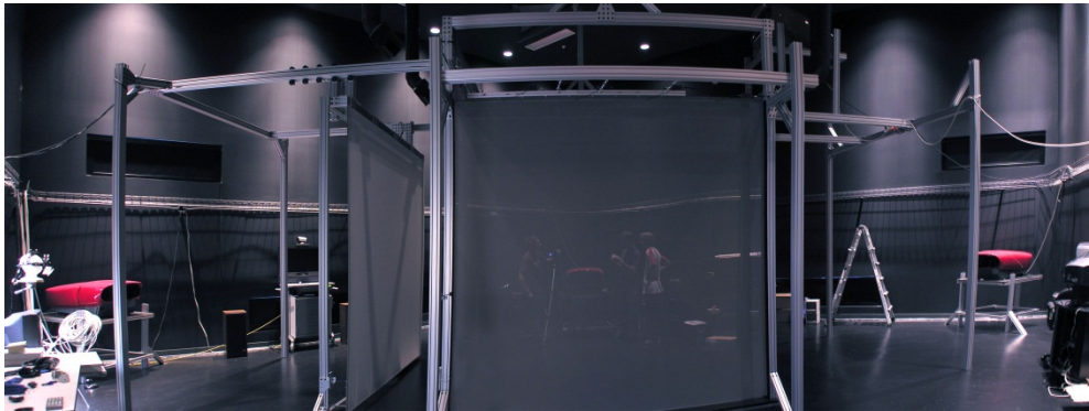
Figure 4. A room-size immersive system where the user stands up in a cube with stereoscopic images retro-projected on its wall to create a very strong sense of presence.
