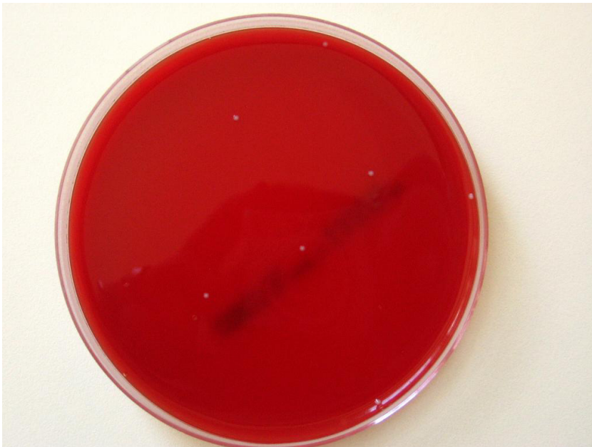
Fig. 7. The bacterial counting test for silver coated wool with E.Coli
