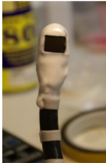
Figure 2. An image of a TEE probe with the EM sensor permanently mounted near the transducer face.
