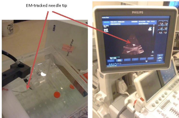
Figure 3. The TEE probe was calibrated by acquiring images of the needle at different orientations. The positions of the EM sensor attached to the TEE probe and the needle are concurrently saved with the image.
