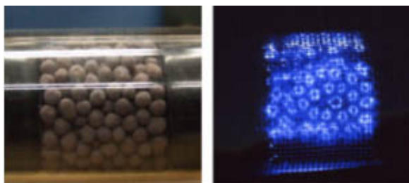
Figure 10. Schematic diagram and its appearance of packed-bed reactor (Photograph: Prof. Takaki group, Iwate University, Japan)[50], [53].
